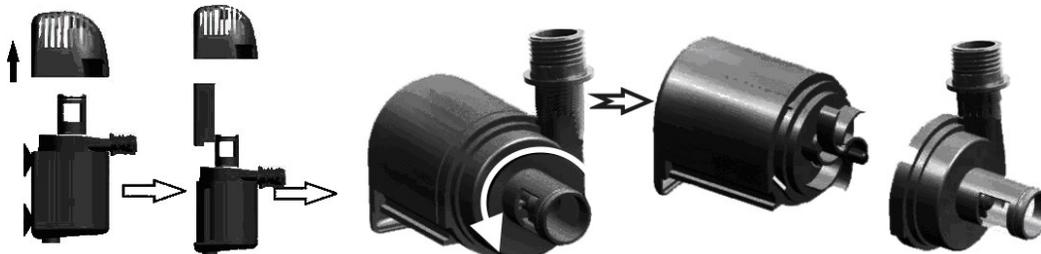
If the pump starts losing power or stops working after operating for a certain time, please clean the pump following the steps below (See the above figures for demonstration):
